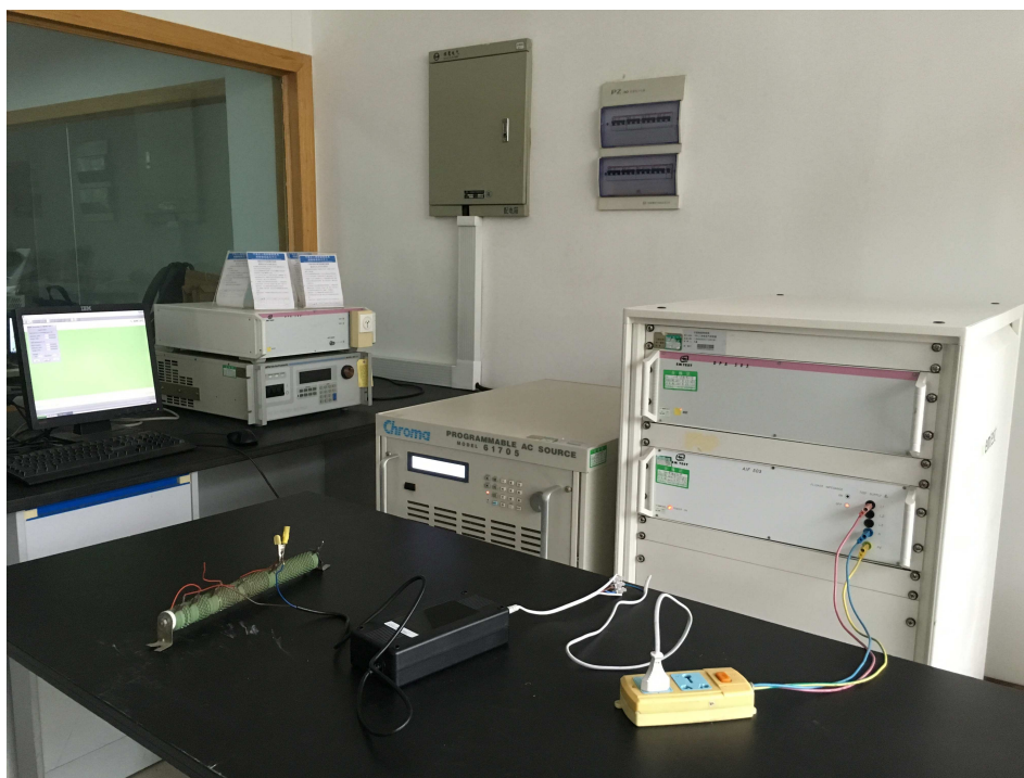
Photograph 2: Set-up for Disturbance Voltage
