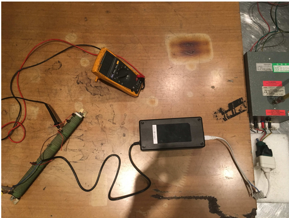
Photograph 6: Set-up for Injected Current
